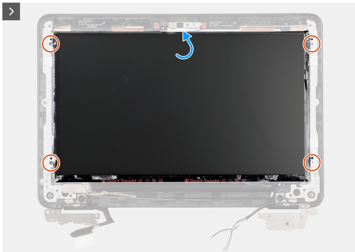
Figure 64. Installing the display panel
